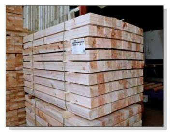
18. Pack of battens stacked in layers as sawn
