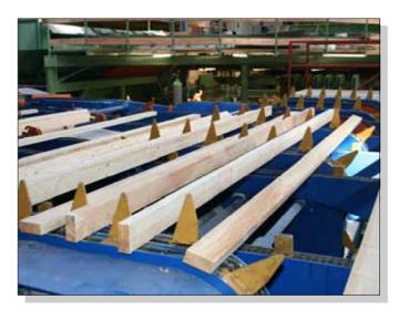
14. Shark fin turner used for fast and convenient inspection
