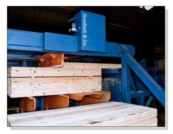
2. Destacking layer longitudinally using push bar
