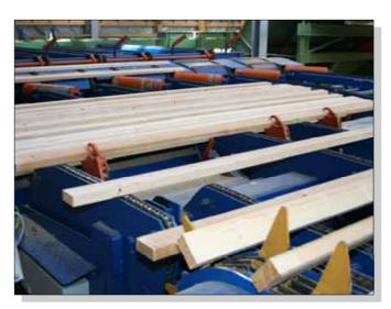
13. Single piece feeder *BCO Speed Feeder* getting a secure grip
