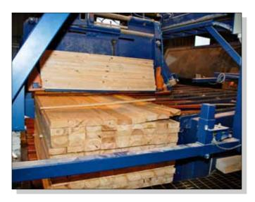
5. Standard stacking machine with stick laying
