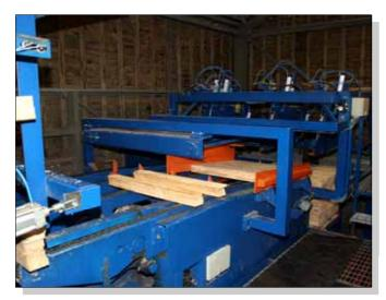
16. Layers being fair-ended while entering high capacity stacking machine.
