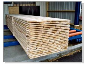
9. Stacking of mixed widths using horizontal spacing – ideal for kiln drying
