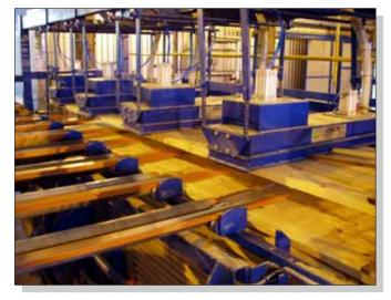
3. Destacking layer transversally using vacuum
