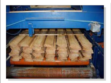
11. Stacking of layers of planks resawn in to slats
