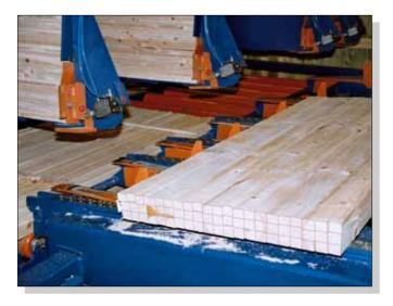
10. Stacking of layers of timber resawn in to battens
